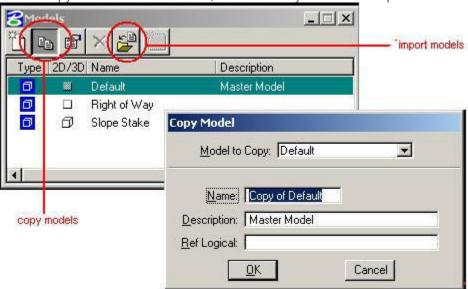
If you just want to copy part of a model, then reference the file interactively and choose the particular model. Once referenced, treat the model like any file and copy any element from the referenced model to the active file.
